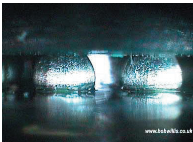
Typical BGA joint with SAC
