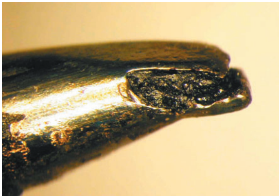
Solder Iron Tip failures when using Lead-free.
