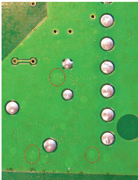
Blistering of solder mask with excessive pot temperatures
