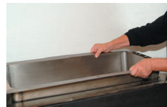
Figure 5. Installation of Solder Pot Liner
