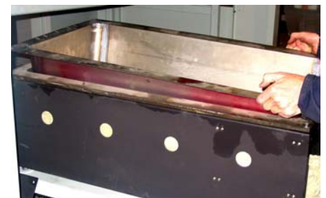
Figure 2. Titanium solder pot liner prevents iron dissolution and increases life of solder pot.
