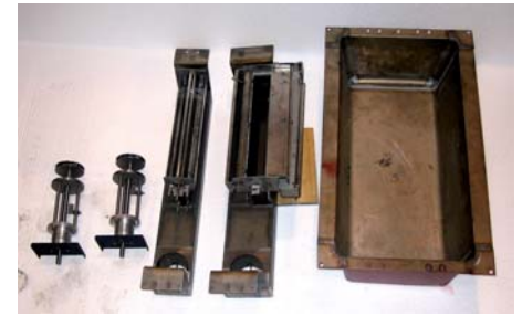
Figure 1. A lead-free retrofit kit with titanium impellers, baffles and solder nozzles.
